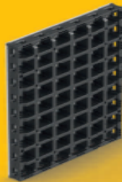
DUO Panels are available in heights of 135 cm as well as 60 cm. With 6 different panel widths ranging from 15 cm to 90 cm, adjustments in 15 cm increments are possible.
